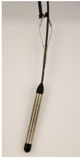
Figure 7-1. Transducer suspended with split mesh cable grip
